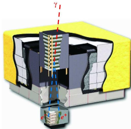
**Fig. 1** The Large Area Telescope (LAT), the main GLAST instrument. An incident gamma-ray enters the detector and produce a  $e^-e^+$  pair, whose tracks and energy are reconstructed in order to derive the direction and energy of the incoming photon.
