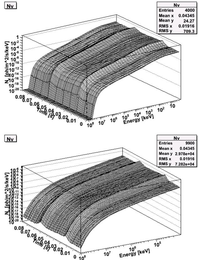
**Fig. 4** Two example of pulsar models given in input to the *PSRShape* model. Above: A Polar Cap phase averaged spectrum from [3]. Below: An Outer Gap phase averaged spectrum from [4]. The sharper cutoff for the Polar Cap is clearly visible
