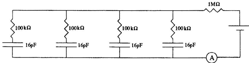
Fig. 1. Electrical model of MSGCs used in the tests.
