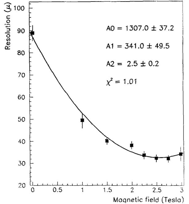
Fig. 2. Position resolution as a function of the magnetic field.
