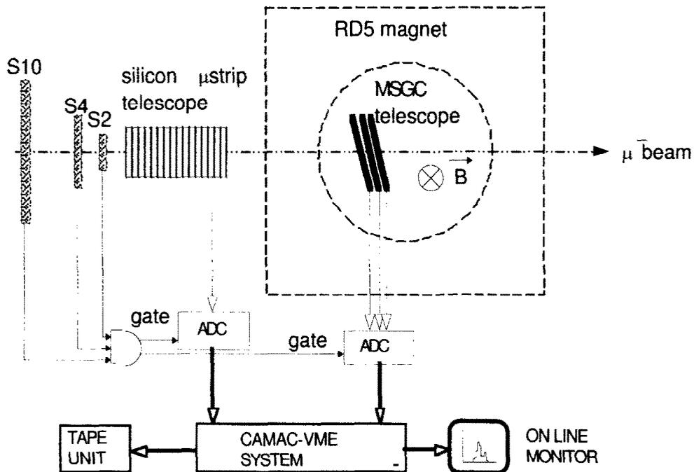
Fig. 12. The general view of the experimental set-up.
