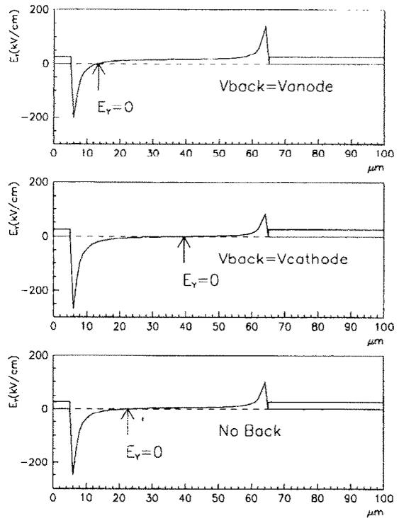
Fig. 6. The vertical component of electric field on the substrate for the bias schemes:  $V_{back} = V_{anode}$ ,  $V_{back} = V_{cathode}$ , no back.
