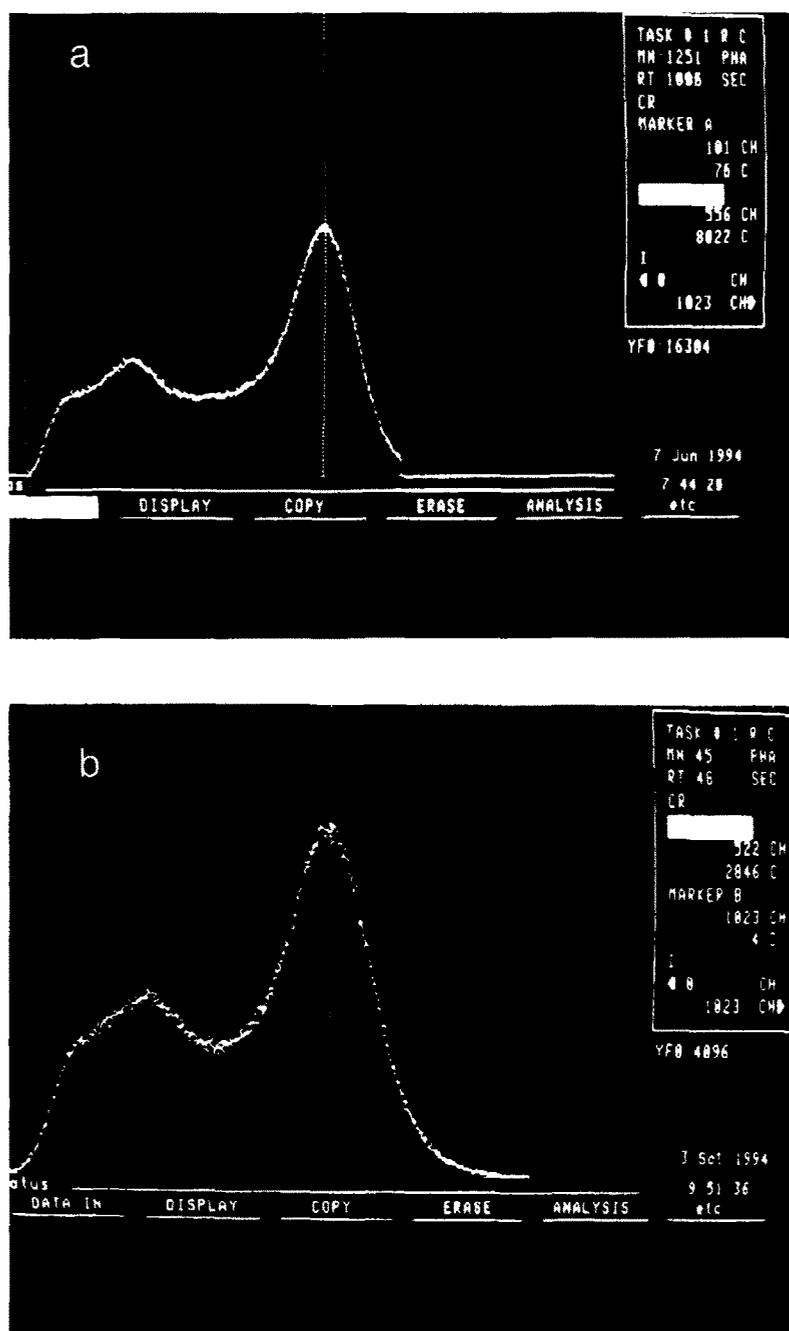
Fig. 11. (a)  $^{55}\text{Fe}$  pulse height distribution at the beginning of the stability measurement under HV.  $V_{\text{cathode}} = -570$  V,  $V_{\text{drift}} = -3000$  V. (b)  $^{55}\text{Fe}$  pulse height distribution recorded 3 months after that one of (a).
