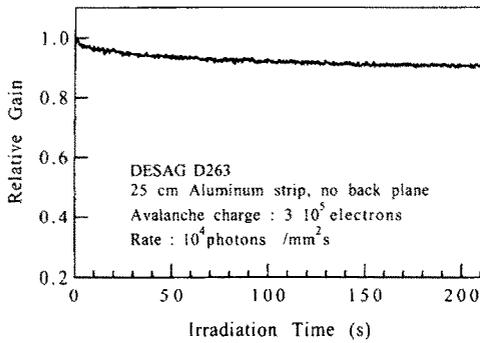
Fig. 4. Short-term measurement of the gain stability.
