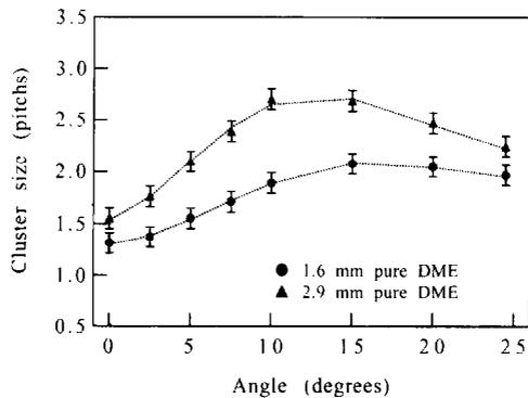
Fig. 14. The dependence of the cluster size on the track angle.
