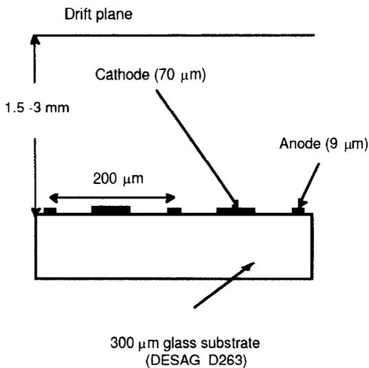
Fig. 1. A cross section of the detector.
