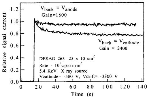
Fig. 5. Time dependence of the gain for the two different bias schemes.
