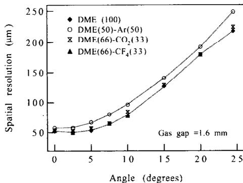
Fig. 15. The dependence of the spatial resolution on the incidence angle of the track for different gas mixtures.
