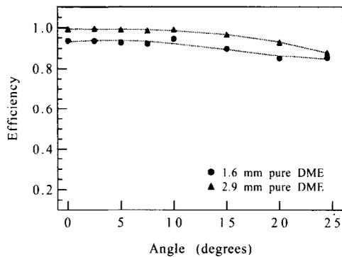
Fig. 18. The cluster detection efficiency in pure DME for 1.6 and 2.9 mm gas gap.
