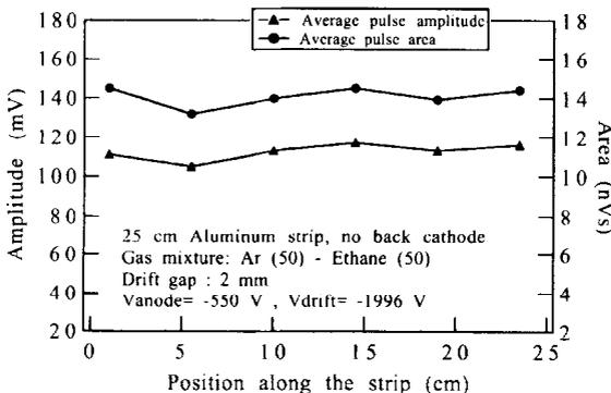
Fig. 8. Uniformity of response along the 25 cm strip.
