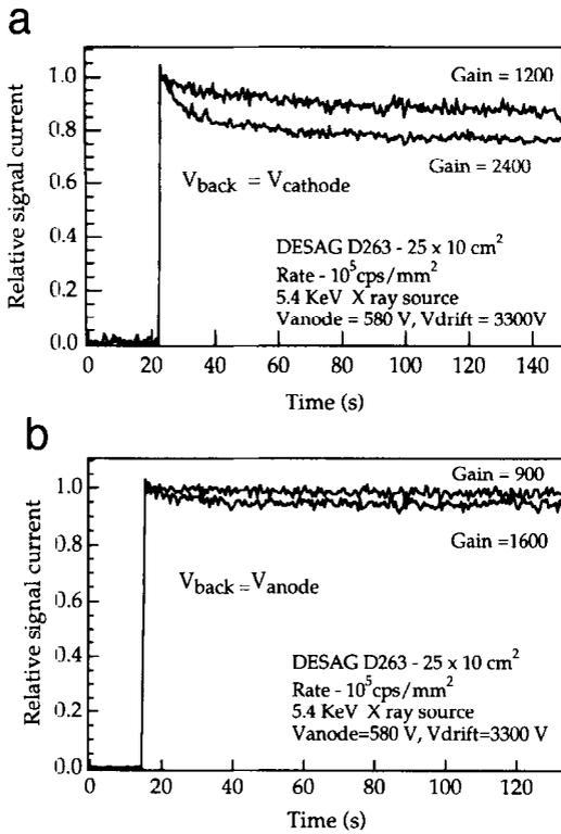
Fig. 7. (a) Dependence of charging with gain in the case  $V_{back} = V_{cathode}$ . (b) Dependence of charging with gain in the case  $V_{back} = V_{anode}$ .
