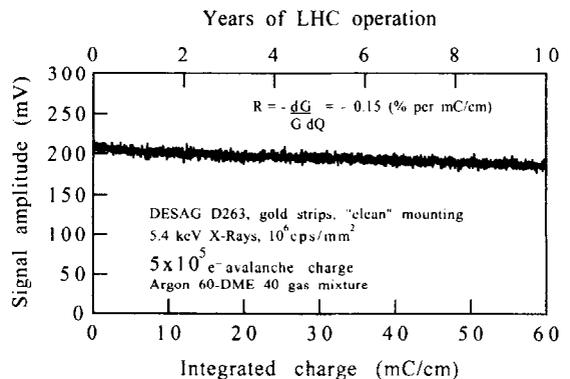
Fig. 10. Very long-term measurement of the gain stability (ageing).
