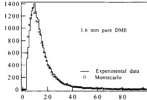
Fig. 16. The pulse height distribution obtained with 1.6 mm pure DME.
