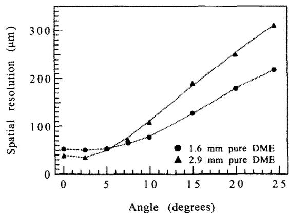
Fig. 13. The dependence of the spatial resolution on the incidence angle of the track for two gas gaps.
