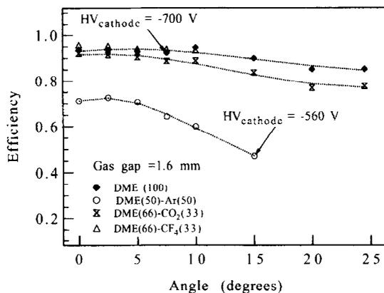
Fig. 19. The detection efficiency for different gas mixtures (gas gap = 1.6 mm).
