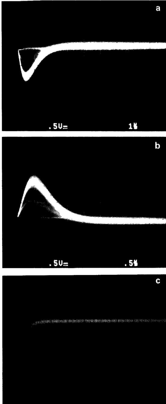
Fig. 7. (a) The anode signal, (b) the cathode signal, (c) the back-strips signal. The source was  $^{55}\text{Fe}$  and the gas filling was argon- $\text{CO}_2$  at atmospheric pressure.
