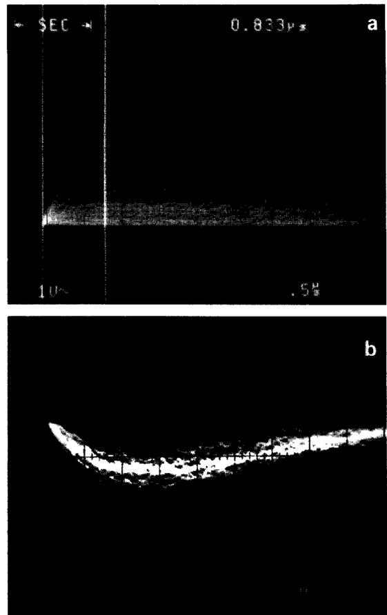
Fig. 9. (a) The signal from the microstrip anodes with a  $^{90}\text{Sr}$  source and a very long ( $\cong 50 \mu\text{s}$ ) differentiation time constant to avoid the problem of ballistic deficit; (b) the corresponding signal from the standard MWPC.
