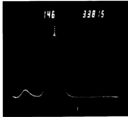
Fig. 8. The pulse height spectrum of the signal of fig.7a. The FWHM of the 6 keV peak is 18%.
