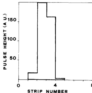
Fig. 11. A typical single-event pulse height distribution on the cathode strips ( $^{55}\text{Fe}$ ).
