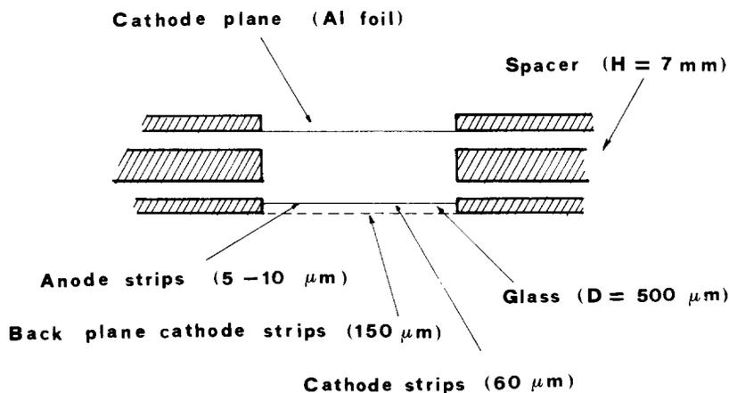
Fig. 1. A cross section of the detector assembly.
