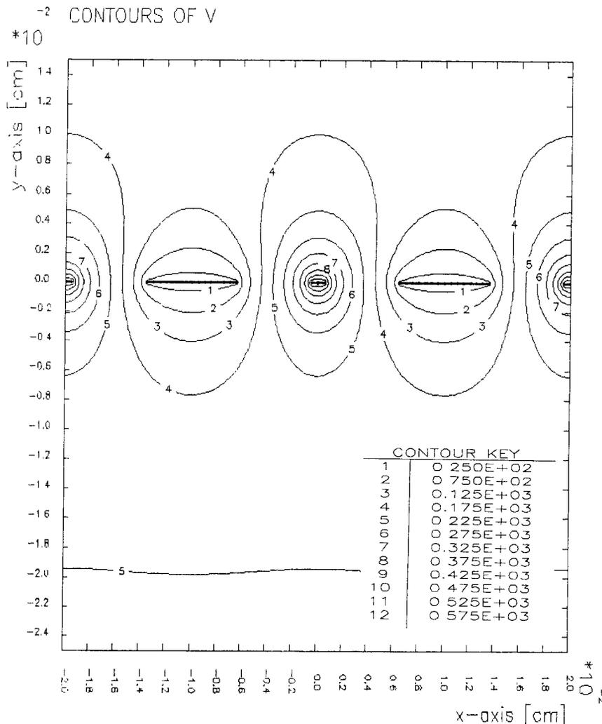
Fig. 3. A detail of the equipotential lines in a region close to the anode strips.
