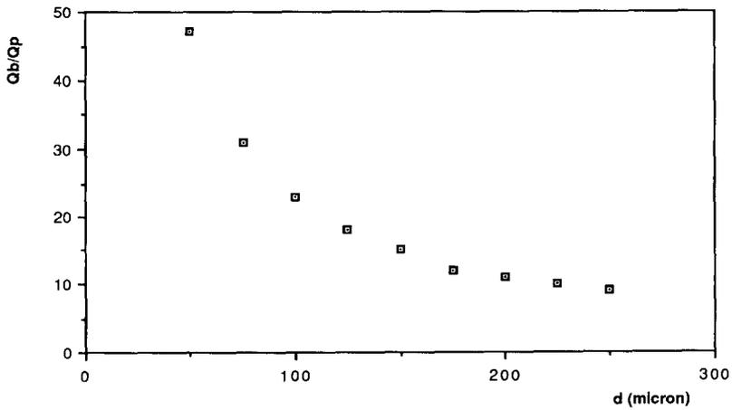
Fig. 6. The ratio between the charge induced on the back strips and the charge induced on the front cathode strips as a function of the effective detector thickness  $d$ .
