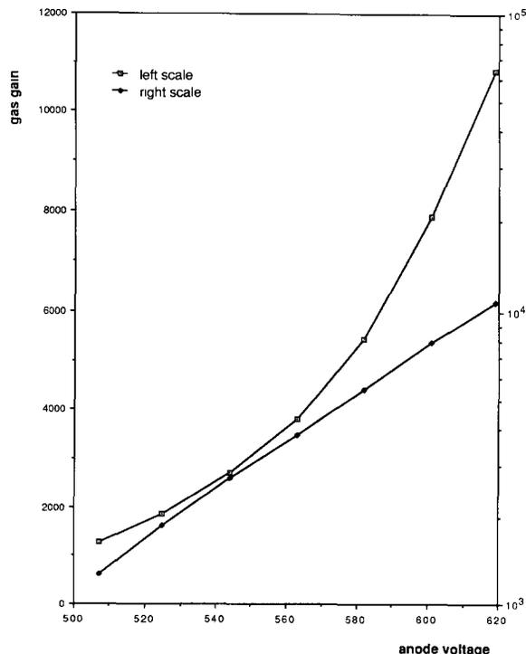
Fig. 10. The gas gain as a function of the potential difference between anode and cathode strips. The gas filling was argon- $\text{CO}_2$  at atmospheric pressure and the source was  $^{55}\text{Fe}$ .
