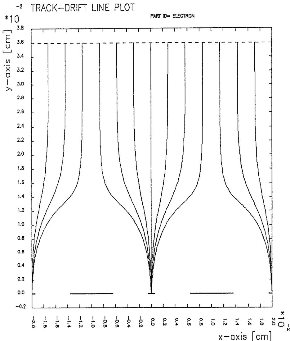
Fig. 4. The drift path for electrons toward the anode strips.
