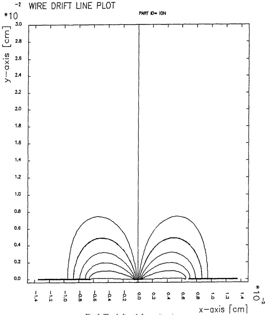
Fig. 5. The drift path for positive ions.
