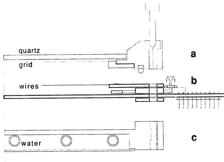
Fig. 4. Cross section of the chamber general assembly: (a) quartz window frame, (b) wires and pads subassembly, (c) back plane and heating system.
