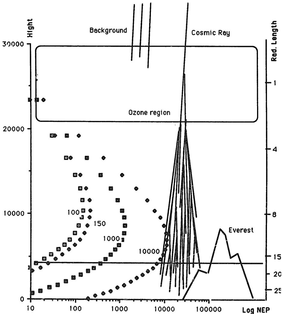
Fig. 1. Schematic view of the measurement principle and several profiles of showers of different energies.
