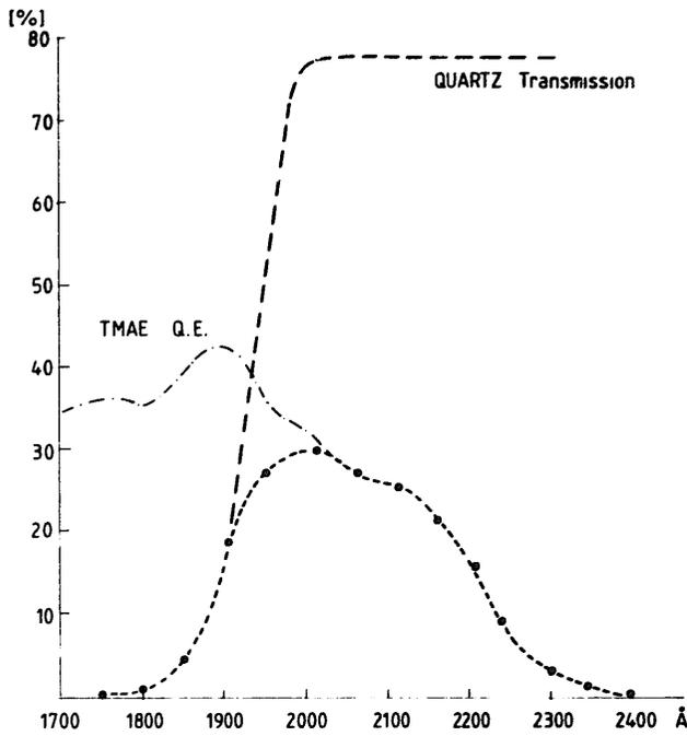
Fig. 2. Quantum efficiency of TMAE and quartz transmission.
