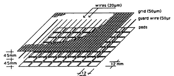
Fig. 3. Basic geometry of the chamber and schematic lay-out of the electrodes.
