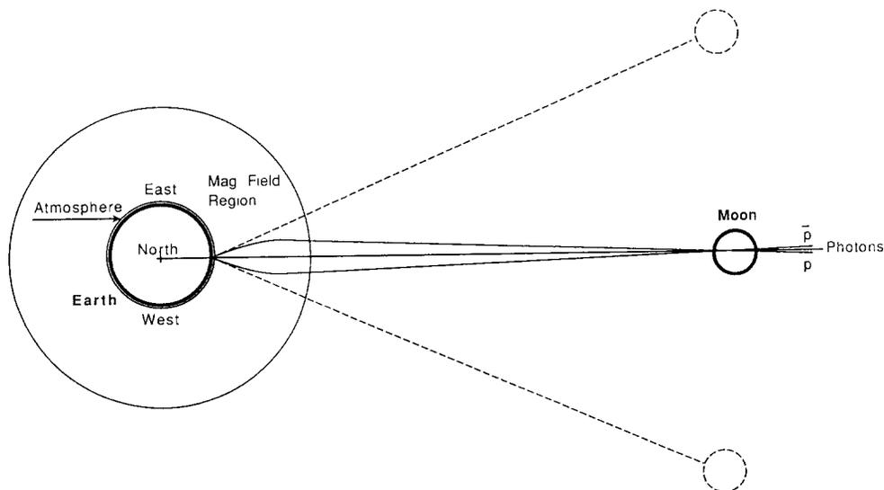
Fig. 4. Schematic illustration of the method of observing the rate decrease due to the shadowing by the Moon of different types of particles. The figure is not to scale.
