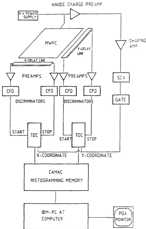
Fig. 1. A schematics of the detector and its associated electronics.
