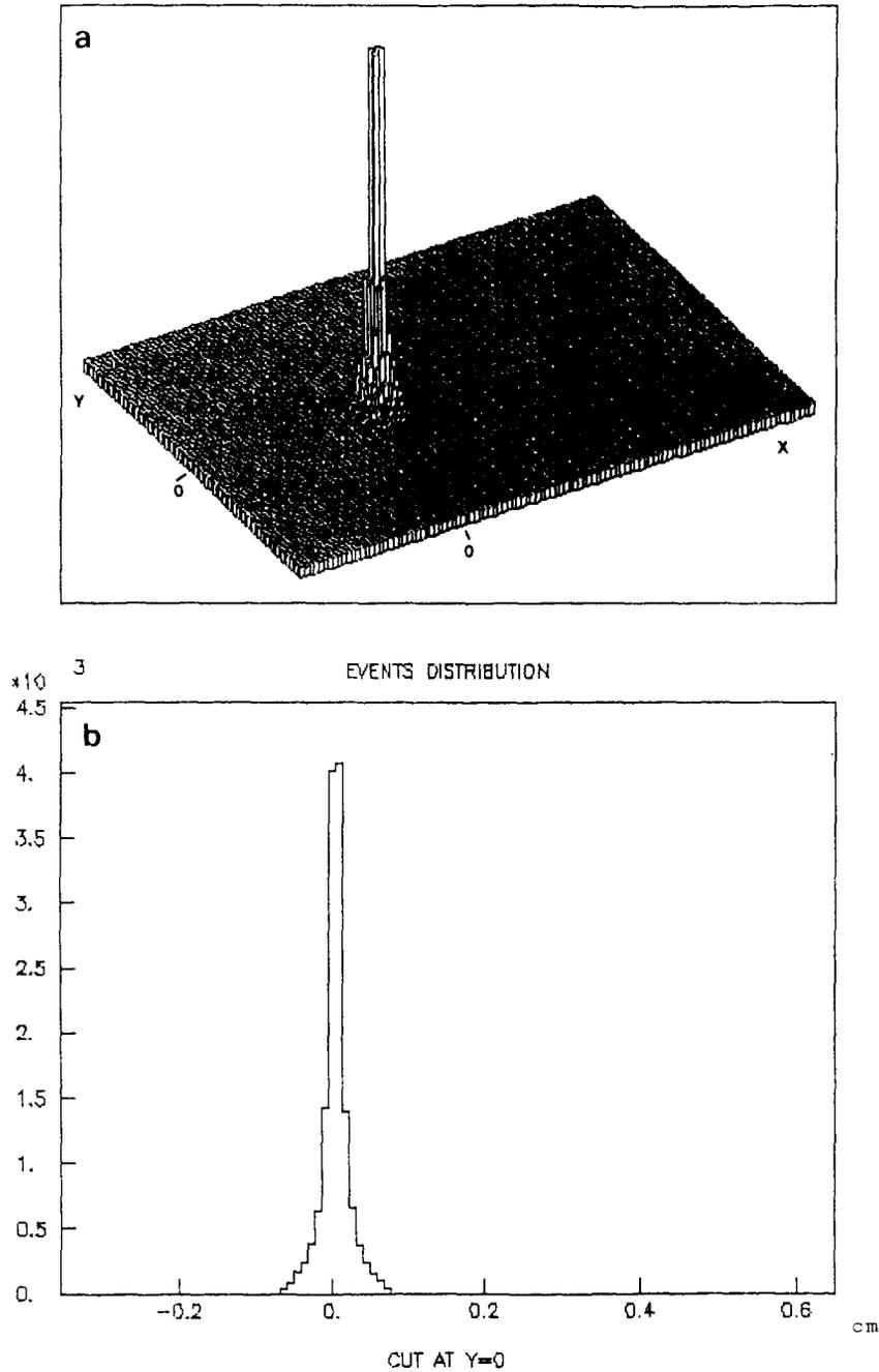
Fig. 6. (a) Scatter plot of the reconstructed events coming from a 70 keV point source placed at 1 m and impinging in the middle of the detector; (b) a cut through the center of the distribution in (a).
