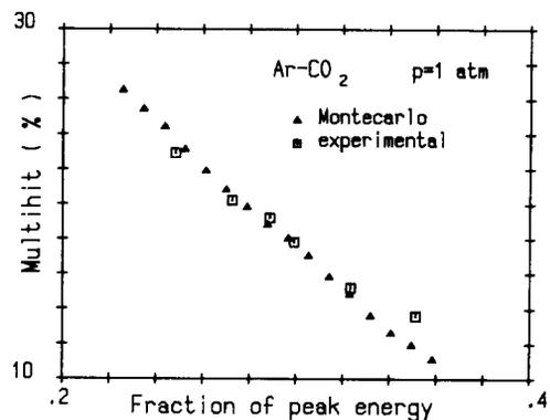
Fig. 5. The number (%) of multihits versus energy threshold (Monte Carlo and experimental).
