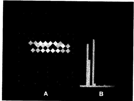
Fig. 4. (a) The reconstructed image of two slits  $100\ \mu\text{m}$  wide,  $1.8\ \text{mm}$  apart, (b) the histogram obtained when projecting the image of (a) along the vertical axis.
