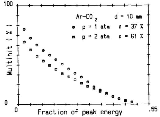
Fig. 8. The multihit fraction in an argon-CO<sub>2</sub> mixture at 1 and 2 atm.
