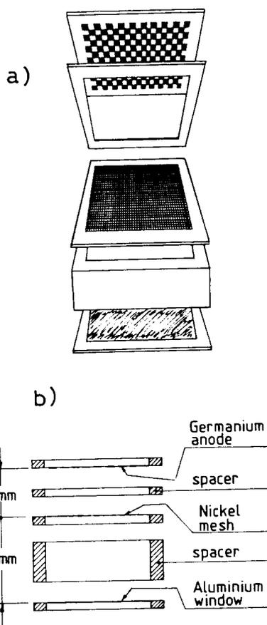
Fig. 1. (a) An exploited view of the detector assembly; (b) a cross section of the detector.
