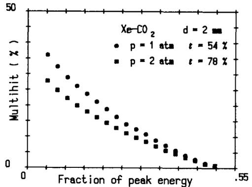
Fig. 9. The multihit fraction in a xenon-CO<sub>2</sub> mixture at 1 and 2 atm.
