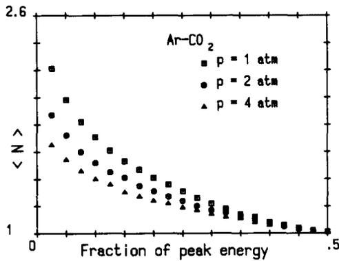
Fig. 6. The mean number of pads with signal over the threshold, i.e. with a charge larger than a preset fraction of the total ionization charge versus the threshold itself, for a drift region 1 cm thick and for different values of pressure in an Ar-CO<sub>2</sub> mixture.
