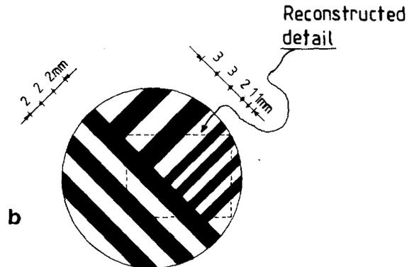
Fig. 2. The reconstructed image of the detail inside the dashed box (a) and  $^3\text{H}$  resolution phantom (b).
