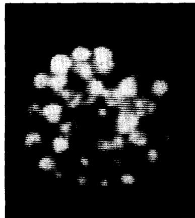
Fig. 3. Reconstructed image of a  $^{14}\text{C}$  disk source made up of several "point sources".
