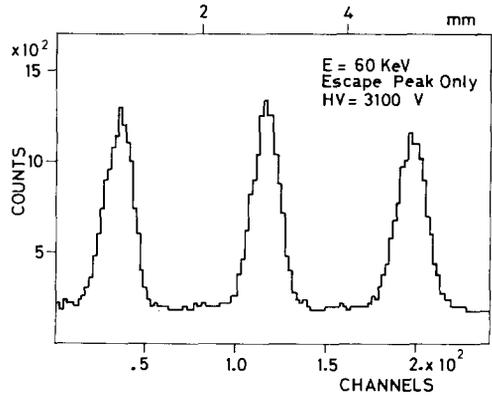
Fig. 9. A wire spectrum obtained with a <sup>241</sup>Am source (59.5 keV). Only the events within the escape peak are accepted.
