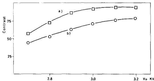
Fig. 8. Curve a): the contrast of the wire pattern as a function of the operating voltage for events within the escape peak, curve b): the same as a), with all the events accepted.
