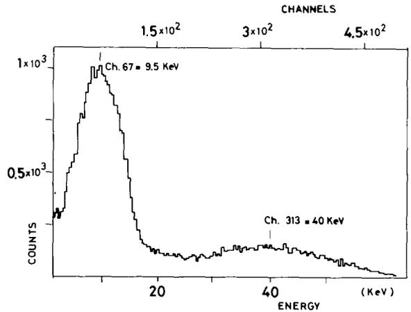
Fig. 4. Anode pulse-height spectrum at 40 keV and 2 atm.
