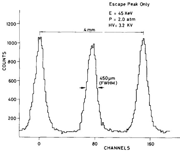
Fig. 6. PHA wire spectrum along the direction orthogonal to the anode wires. Only the events within the escape peak are accepted.
