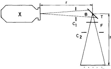
Fig. 1. A scheme of the fluorescent X-ray source: C1: entrance collimator, C2: exit collimator, T: target, F: filter.
