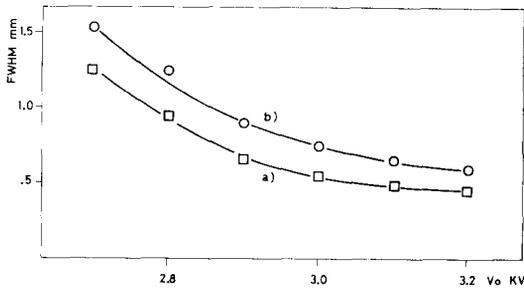
Fig. 7. Curve a): spatial resolution as a function of the operating voltage for events within the escape peak, curve b): the same as a), with all the events accepted.
