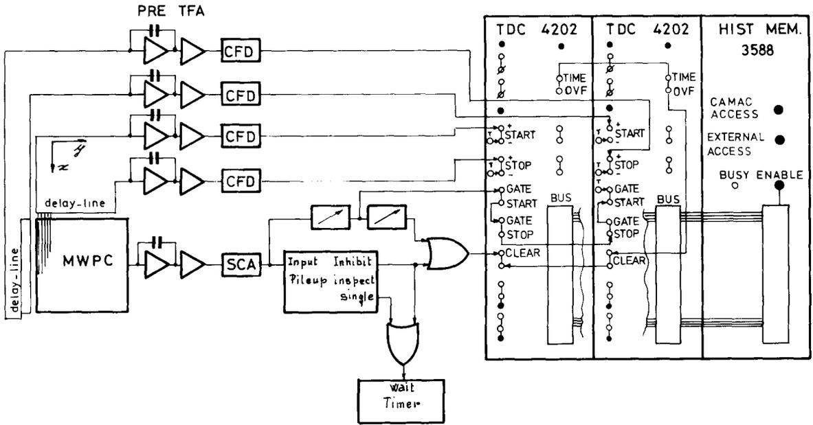
Fig. 3. Block diagram of the position read-out system.
