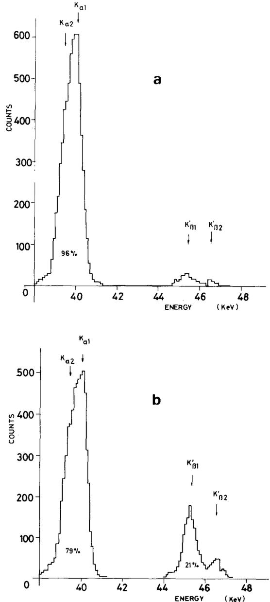
Fig. 2. (a) Spectrum generated by a samarium target with the neodymium filter, (b) the same as (a), without neodymium filter.
