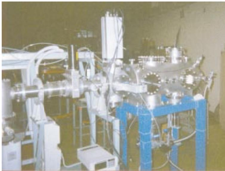
Figure 2: Photo of the ion-beam chamber.
