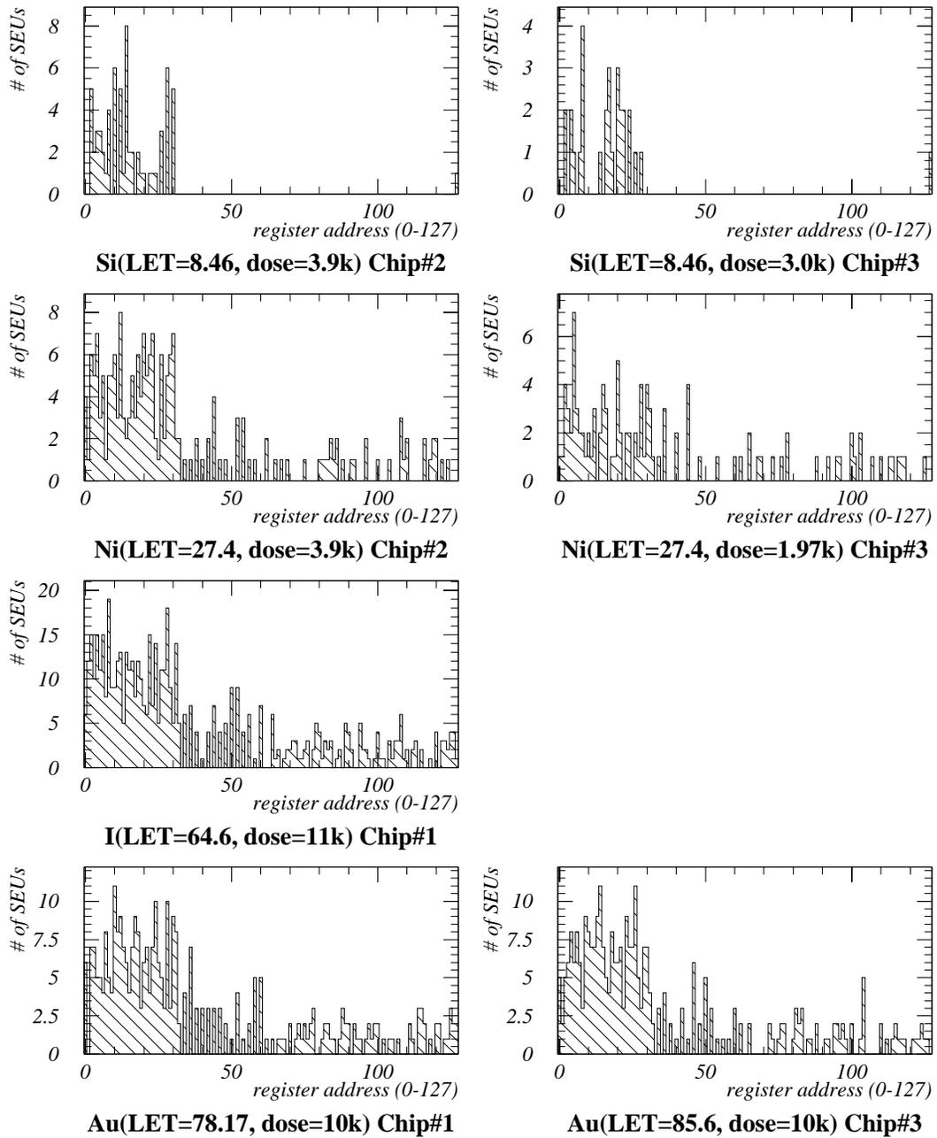
Figure 5: SEU occurrence in each individual cell of 128-bit-shift register block.
