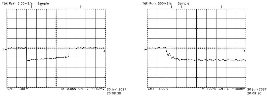
Figure 14: Observed waveforms of simulated latchup signals by (B) current monitor system.
