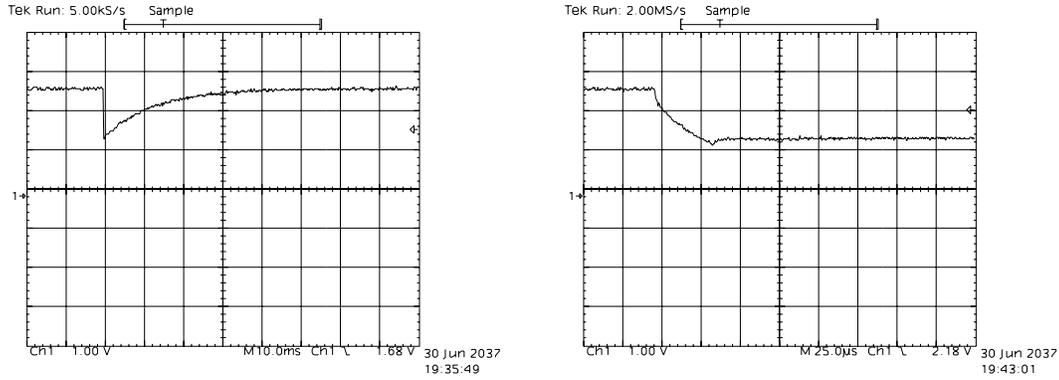
Figure 13: Observed waveforms of simulated latchup signals by (A) voltage monitor system.
