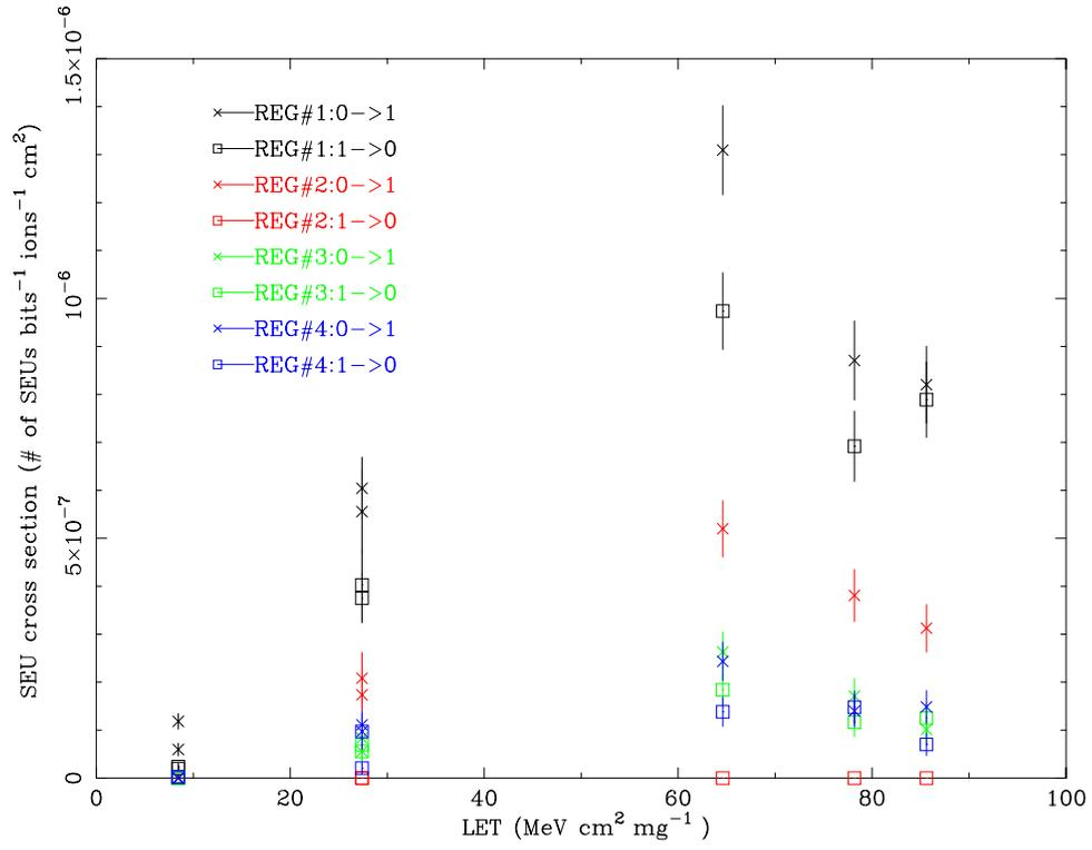
Figure 9: SEU cross section—LET relation (linear-scale plot).
