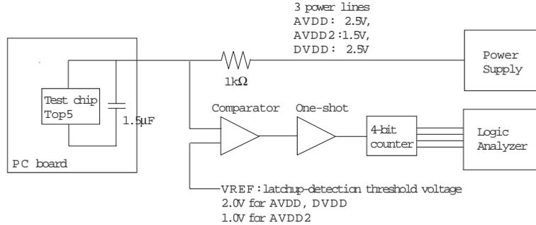
Figure 3: Schematic of latchup detection circuit
