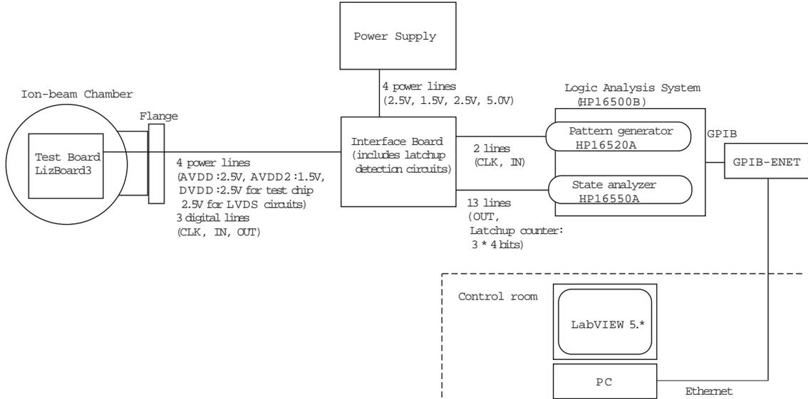
Figure 4: Configuration of test system at the INFN-LNL heavy-ion beam facility
