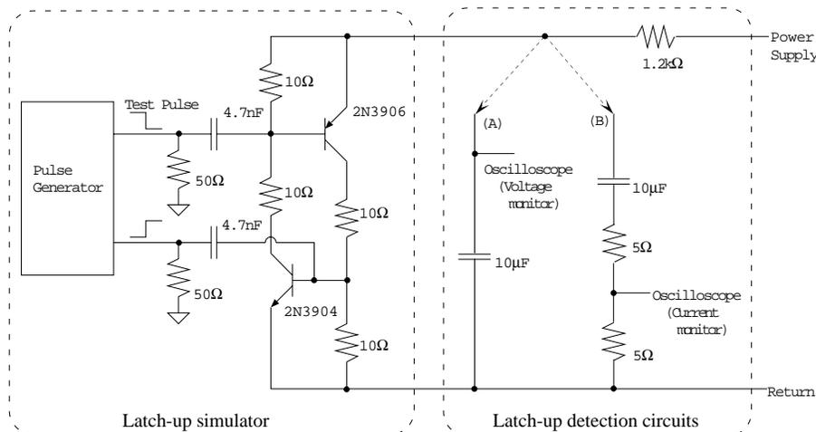
Figure 12: Schematic diagram of latchup simulation circuit and latchup detection systems.
