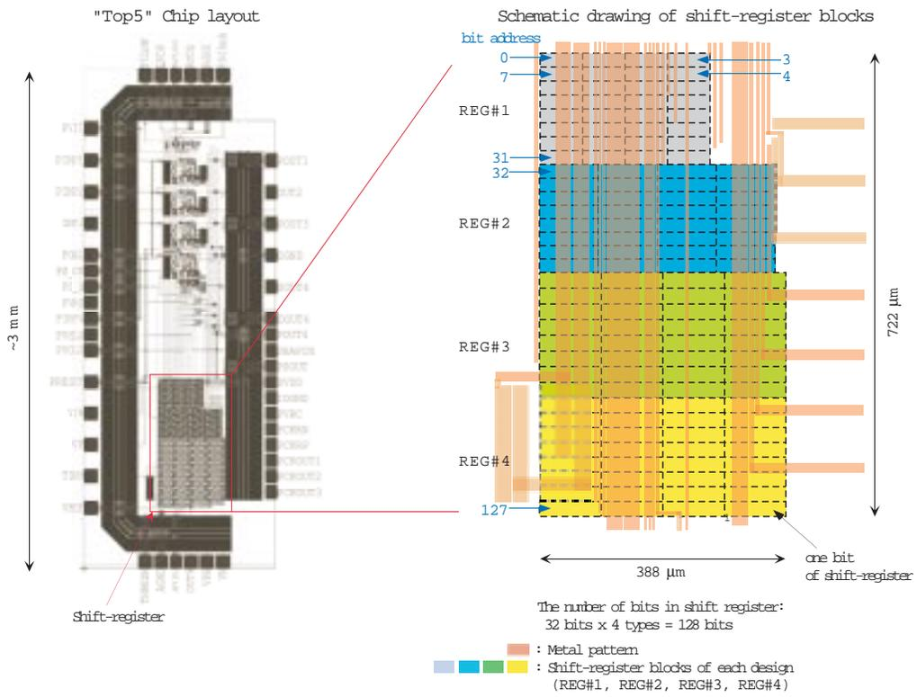
Figure 1: "Top5" chip layout and schematic drawing of the 128-bit shift-register on the chip
