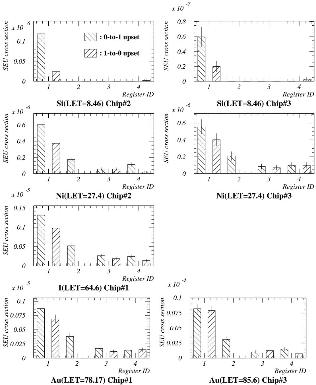
Figure 6: SEU cross section for each register design and transition mode:
