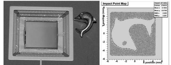
Figure 5. Image of an ear ring done with a detector based on chip of generation II and processed with the reconstruction of the impact point
