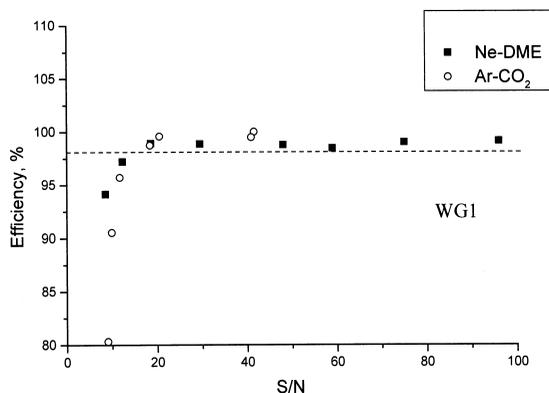
Fig. 10. Efficiency vs.  $S/N$  for WG1.
