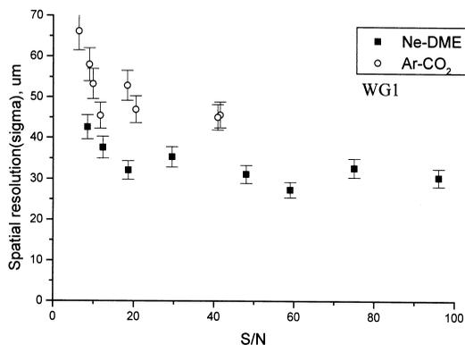
Fig. 12. Spatial resolution vs.  $S/N$  for WG1.
