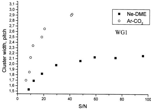
Fig. 13. Cluster width vs.  $S/N$  for WG1.
