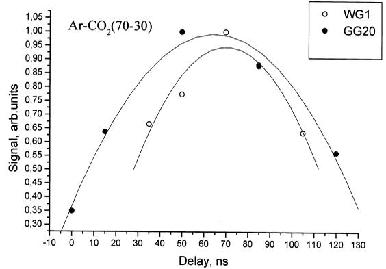
Fig. 8. Delay curves for Ar–CO<sub>2</sub>.
