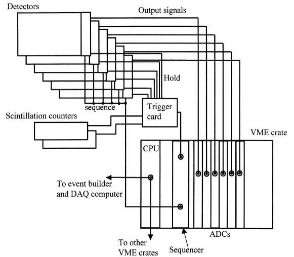
Fig. 3. Data acquisition system.
