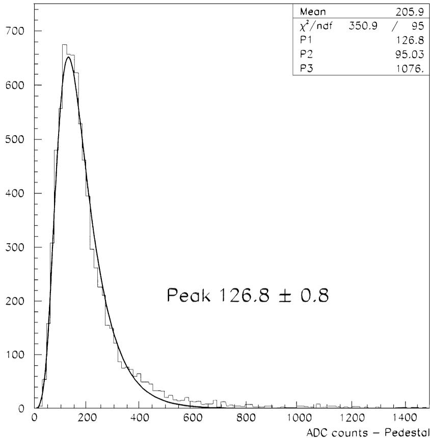
Fig. 1. Cluster charge at  $V_{\text{cathode}} = 530$  V,  $V_{\text{drift}} = 3000$  V, 25% Ne–75% DME gas mixture.
