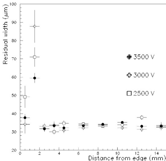
Fig. 2. Standard deviation of the residual distribution as a function of the distance from the chamber edge, at  $V_{\text{cathode}} = 540$  V, 25% Ne–75% DME gas mixture, for different conditions of the drift voltage.
