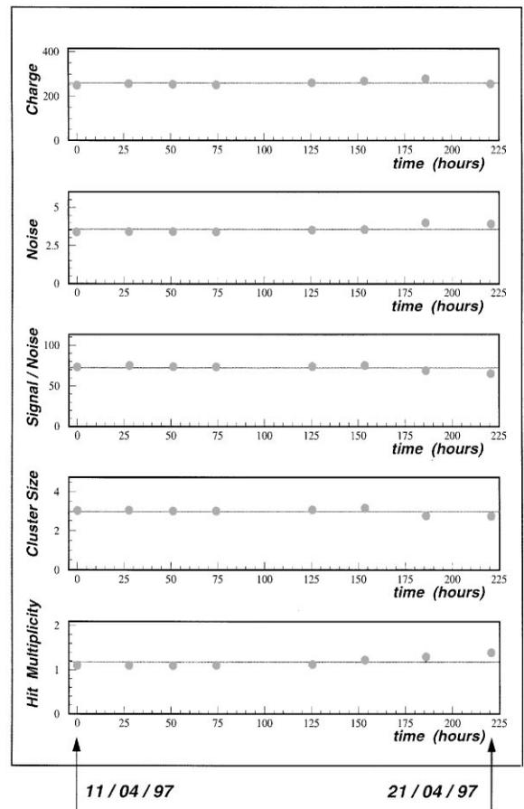
Fig. 4. Stability study for a MSGC chamber. All variables are plotted for the 225 h of running time; the data were recorded in low-intensity runs.
