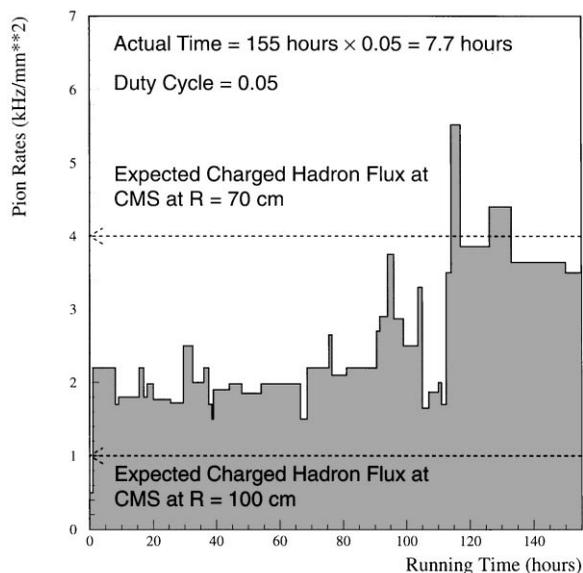
Fig. 1. Average particle rates measured by a  $0.5 \times 0.5 \text{ cm}^2$  counter set close to the region of maximum beam intensity as a function of integrated running time.
