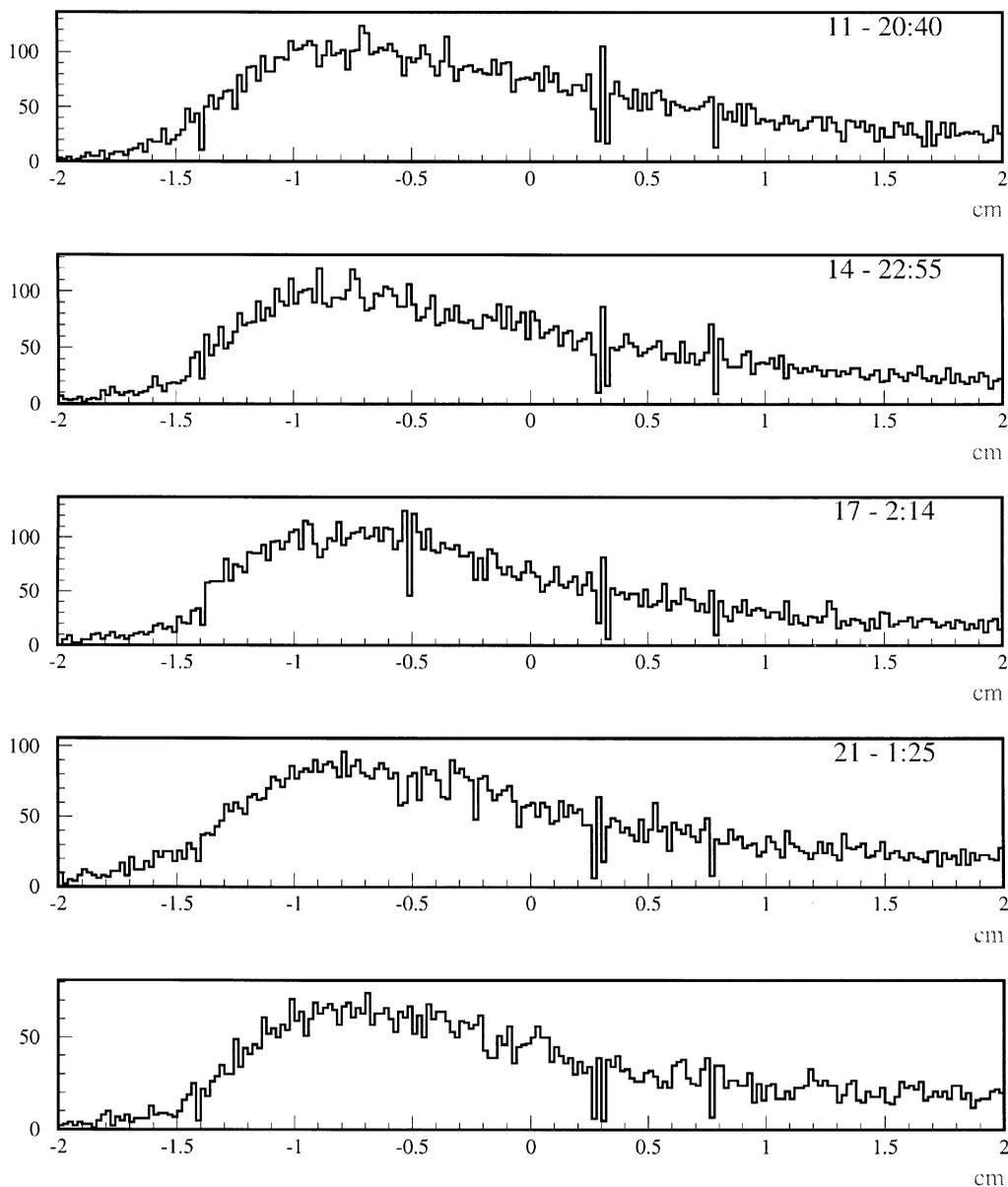
Fig. 3. Beam profile seen by a MSGC detector from the beginning (first plot) to the end (last plot) of the test. No dead or inefficient strip could be detected.
