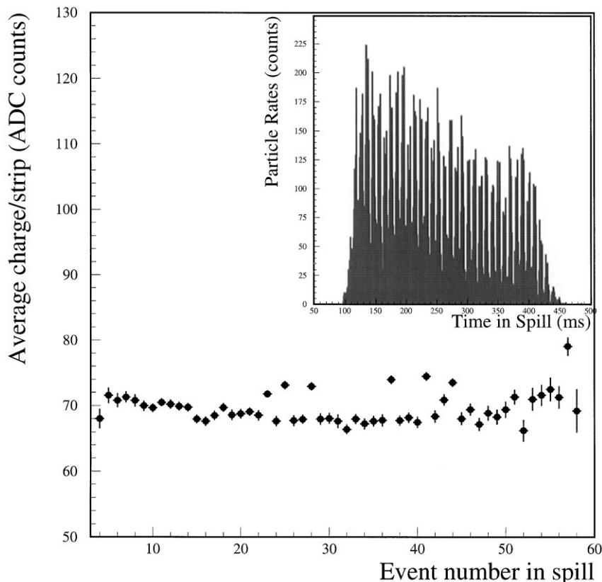
Fig. 2. Most probable value of the total collected charge normalised to the total number of fired strips as a function of the event number in spill. The substrate resistivity is  $1 \times 10^{16}$   $\Omega/\text{cm}^2$ . The inset shows the instantaneous rates recorded by a  $0.5 \times 0.5$  cm<sup>2</sup> counter aligned to the beam profiles maximum (bin = 1 ms) during the same period.
