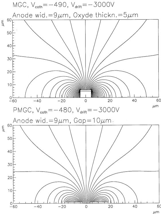
Fig. 2. Electric field maps for an MGC and for a PMGC.
