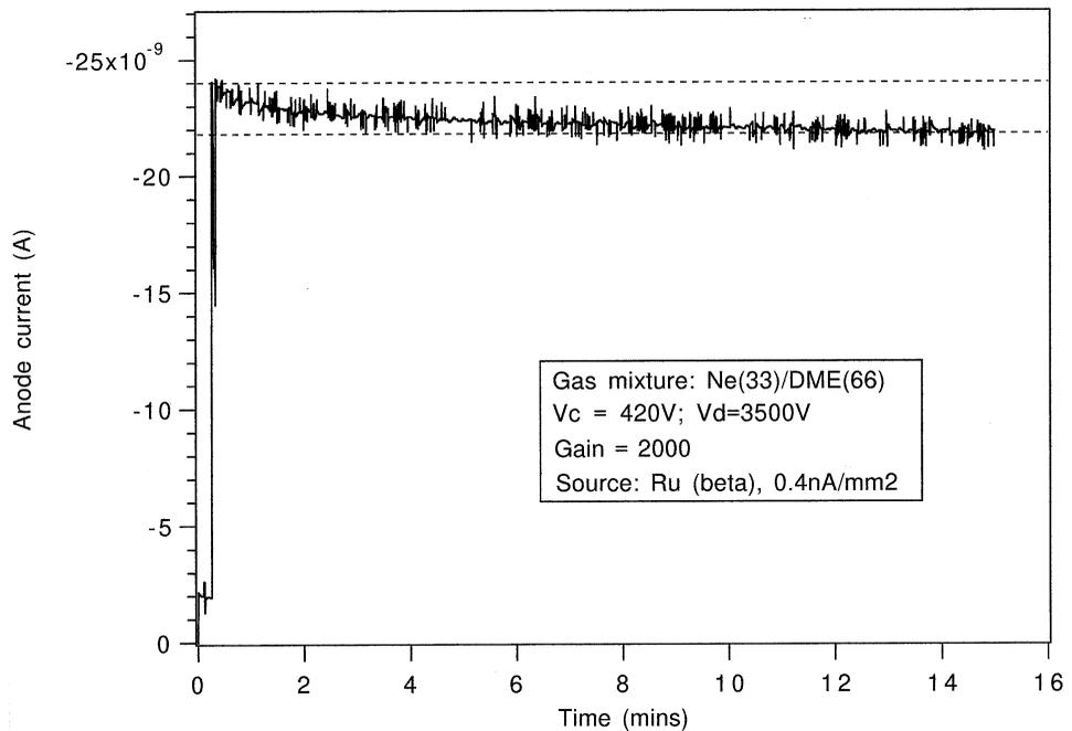
Fig. 5. Time development of charging effect for a PMGC with gap  $10\ \mu\text{m}$ .
