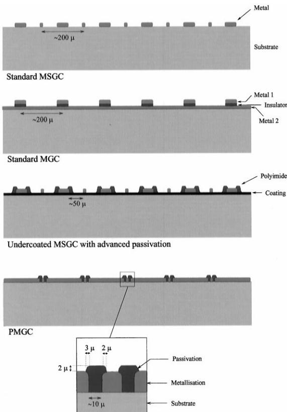
Fig. 1. Comparison of various types of micro-detectors.
