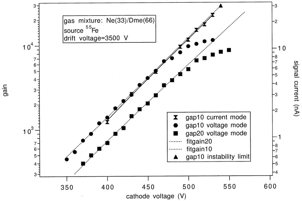
Fig. 4. Gain curves for PMGCs with two different gap widths.
