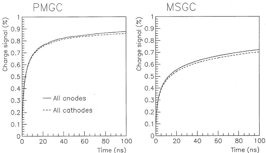
Fig. 3. Percentage of signal charge collected as a function of time for (a) a PMGC and (b) an MSGC.
