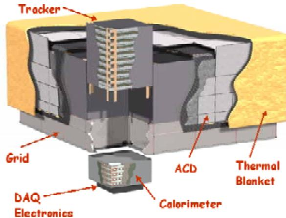
Figure 2. The LAT instrument components
