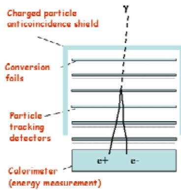
Figure 1. Principle of photon detection in GLAST.
